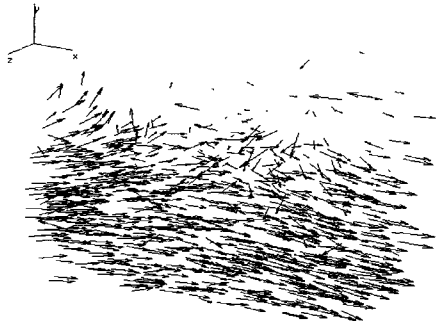
Fig. 12 Three-dimensional vector field around the cylinder at ( t = t_1 )
