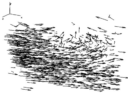
Fig. 13 Three-dimensional vector field around the cylinder at ( t = t_1 + 9/60 sec)
