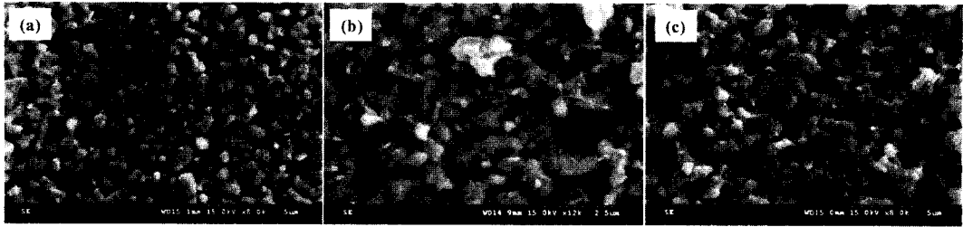
Fig. 6. Microstructure of glass-ceramic produced at different glass contents at 950°C:(a) 5wt%, (b) 10wt%, (c) 15wt%.
