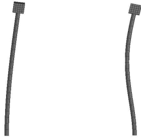
a) 1st mode (7.2Hz) b) 2nd mode (115.3Hz) Fig. 3 Natural modes of the lumped mass model.
