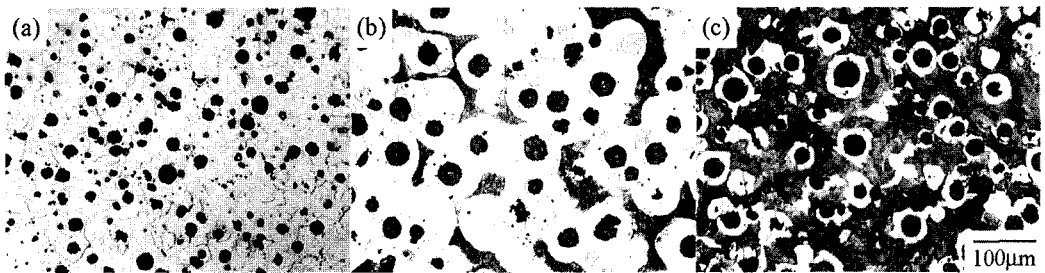
Fig. 3. Optical micrographs of DCI with different chemical compositions. (a) D1M (b) D2M (c) D3M
