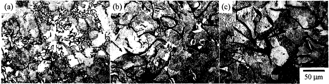
Fig. 5. Optical micrographs of G2(CE:4.049) with various cooling rates. (a) G2S (b) G2M (c) G2L
