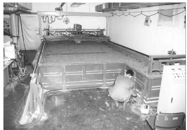
Fig. 1. Soil bin containing cohesive soil of bentonite-water mixture.
