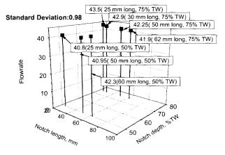
Fig. 5. Relationship among the length, depth and flow rate of the part through wall defects
