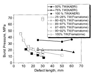
Fig. 4. Effect of the defect length on the burst pressure
