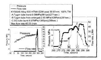
Fig. 6. Burst behavior of a through wall defect tube in a slow pressurization
