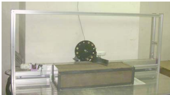
Fig. 2. Photo of system for analyzing motion characteristics of rotary blade.
