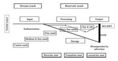
Fig. 5. Dynamics of turbid water after the monsoon rainfall in Hoingsong Reservoir applicable selective withdrawal discharge. WG: watergates, SWT: selective withdrawal tower.
