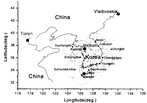
Fig. 5. Locations and coverages of DGPS beacon stations of Korea.
