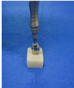
Fig. 9. Automalleting 10sec, 10times every a minute
