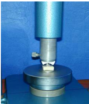
Fig. 8. Cement with Cavitec under 5Kg vertical load,1min
