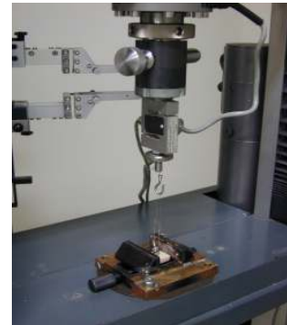
Fig. 10. Measure the tensile strength with UTM
