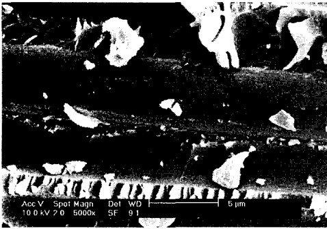
(b) fractured Gr/Ep UD specimen at -150°C
