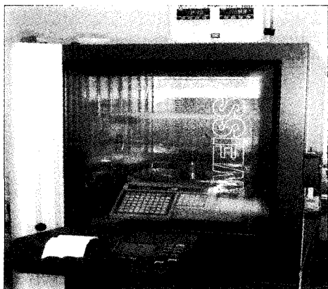
Fig. 6 Damp heat, stability state test
