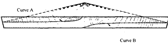
Fig. 7 Drawing of paths of zero contact points
