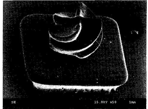
Fig. 10 SEM image of a helical gear fabricated with epoxy composite
