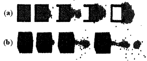
Fig. 9. Simulation for nanojets with (a) \alpha_{AB}=1 and (b) \alpha_{AB}=0.1 .
