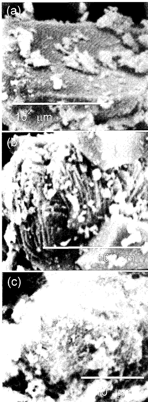
Fig. 8. SEM pictures of C_4AF hydrated in CaSO_4 \cdot 2H_2O - Na_2Si_2O_5 saturated solution for 24 h: (a) surface where no hydrates formed, and (b) and (c) surface where hydrates formed.
