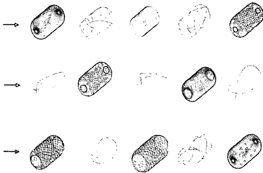
Fig. 10 Winding sequence for composite thickness improvement.
