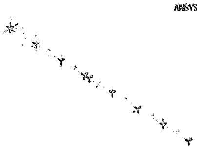
Fig. 12 Simplified engine model using the beam element
