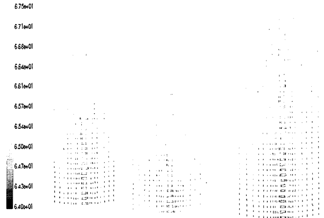
Fig. 6. Winding temperature distribution with the flow rate of 7L/min.
