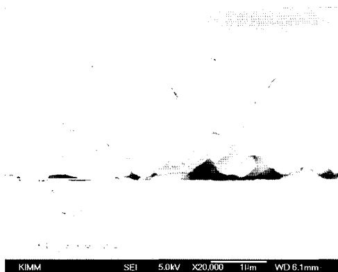
Fig. 7. Cross-sectional view of YBCO thin film prepared by multiple coating method.
