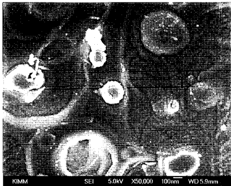
Fig. 6. Microstructure of YBCO thin film prepared by double coating.
