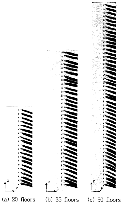
Fig. 4 Flow pattern of the hot air.
