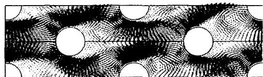
Fig. 4 Flow around tube banks
