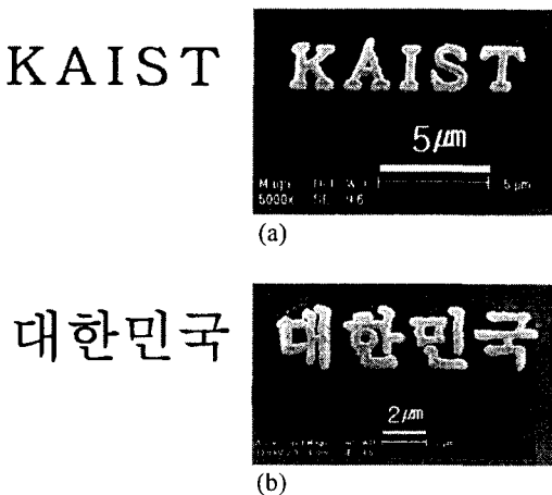
Fig. 7 SEM image of replicated letters of (a) 'KAIST' and (b) '대한민국'
