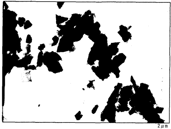
Fig. 5. Representative transmission electron microphotograph of pyrophyllite crystals.
