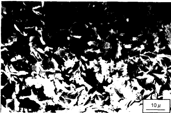
Fig. 4. Characteristic scanning electron microphotograph of pyrophyllite particles.
