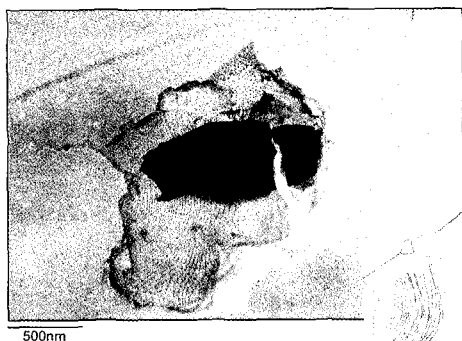
Fig. 7. Surface microtopographies of pyrophyllite crystals collected from the Gussi deposit. Malformed circular step patterns with comparatively regular separations between the neighboring steps.
