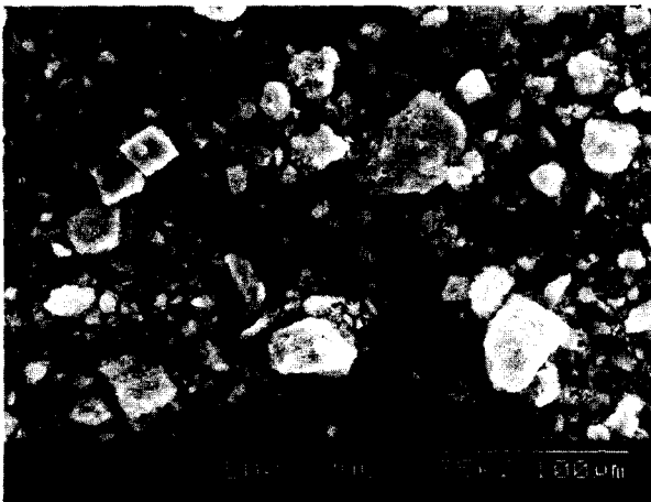
Fig. 11. SEM Photograph for the precipitate resulted from apatite dissolution.
