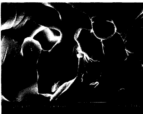
Fig. 5. SEM micrograph of hydroxyapatite precipitate heated at 1250°C; 0.174 M.
