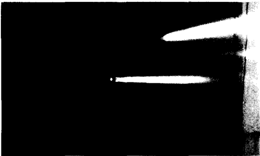
Fig. 3 Typical photographic view of a unielement thrust chamber under firing
