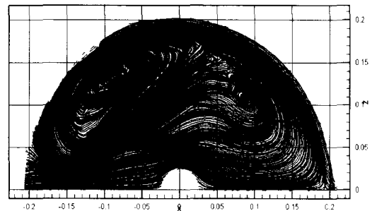
Fig. 15 Streamline pattern on constant y plane ( y=0.02m ) in the LOX manifold of injector modeling
