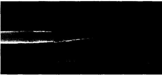
Fig. 8 Machined shape under applied voltage 4.1 V, electrolyte 1.5 M \text{H}_2\text{SO}_4 , and machining time 240 sec
