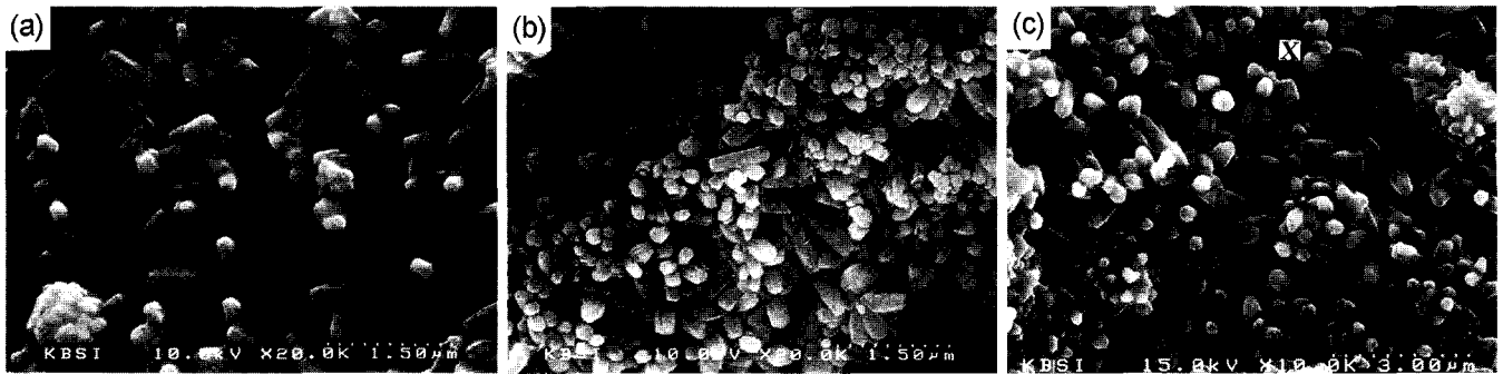
Fig. 9. SEM photographs of the products prepared by hydrothermal reaction of \alpha -TCP at 100°C for (a) 1, (b) 3, and (c) 5 h.
