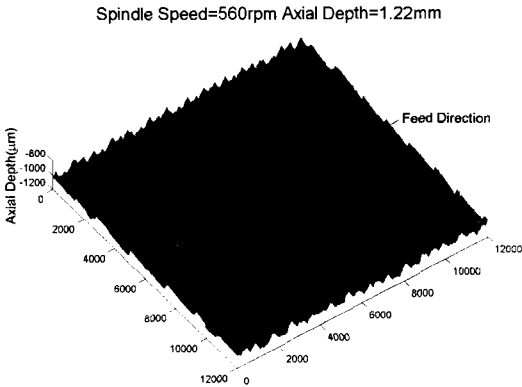
Fig. 11 Measured surface profile without chatter
