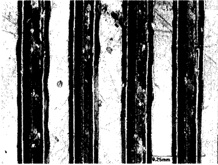
Fig. 7 Front view of machined grooves on polycarbonate (0.67 mm/s, 2 μm)
