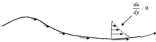
Fig. 6 Description of frictional force mechanism by trochoidal motion
