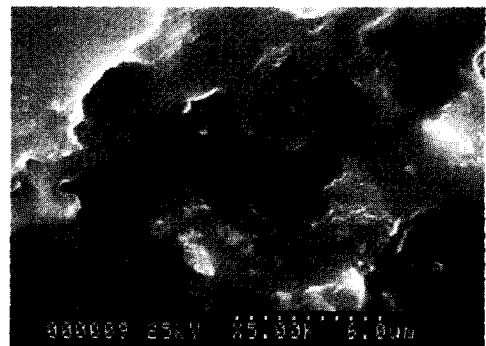
Fig. 7 SEM picture of elasticity style epoxy to which modifier 70 [phr] is added.
