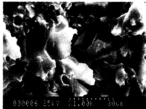
Fig. 6 SEM analysis of elasticity style epoxy to which modifier 35 [phr] is added.
