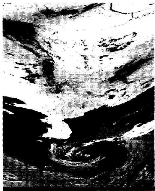
Fig. 7. Images showing the impact of dummy scans at the scene start (bottom). Date of the scene is 20030808 on path 221.
