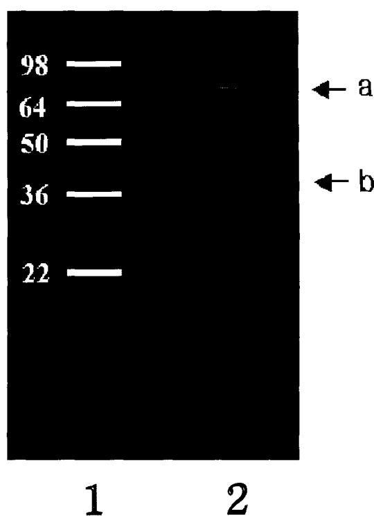
Fig. 6. Gelatin zymography of the culture supernatant. The sample was prepared from a culture broth harvested at 142 hrs after induction. Lane 1; Standard marker, Lane 2; Concentrated culture supernatant (20 \times ). Arrows a and b describe the proteolytic activity of the culture supernatant.
