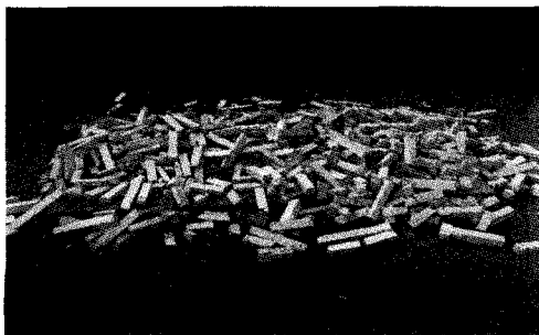
Fig. 18. Result of blasting demolition for scaled model #1
