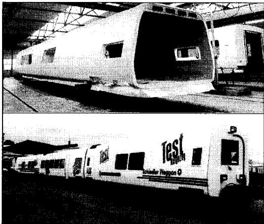
Fig. 1 Carbody structure of tilting train made of composites.
