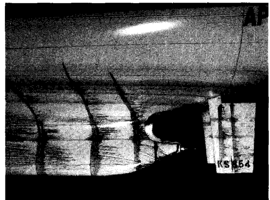
Fig. 8 Paint streaks on KRISO 15,000TEU container ship model with propeller rotating
