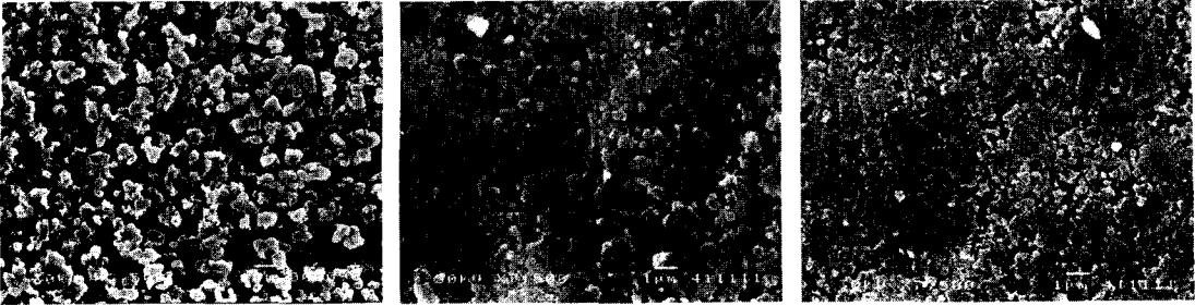
Fig. 4. SEM micrographs of Al-Si and Al-Si-Ni-Ce alloy bar extruded from -25 \mu\text{m} powders at 400^\circ\text{C} and an extrusion ratio of 10 : 1. (a) \text{Al}_{81}\text{Si}_{19} , (b) \text{Al}_{78.5}\text{Si}_{19}\text{Ni}_2\text{Ce}_{0.5} , and (c) \text{Al}_{73}\text{Si}_{19}\text{Ni}_7\text{Ce}_1 .
