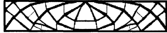
(b) Using the checkerboard-free filter followed by the member-sizing filter ( T_{r_s}^s \circ T_{1.1h}^m )
