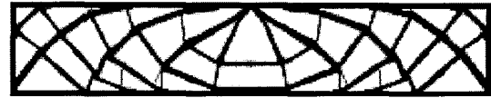
(c) Using the member-sizing filter followed by the checkerboard-free filter ( T_{1.1h}^m \circ T_{r_s}^s )
