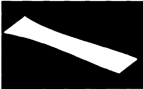
Fig. 10 Beam shape which maximizes fundamental natural frequency
