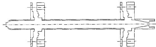
Contraction section Straight section Diffuser section
