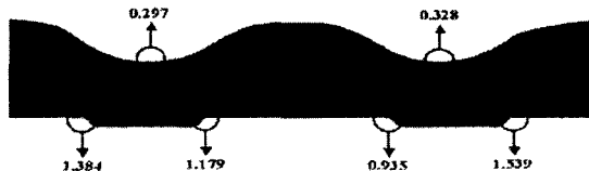
Fig. 13 True stress distribution (Type A)
