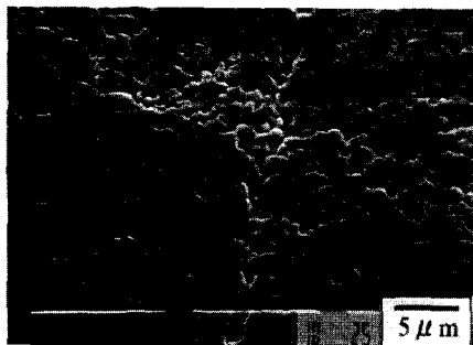
Fig. 3 Alloy surface of the Fe-25Cr steel after pretreatment at 973K in N 2 -0.1%SO 2 (the scale formed during pretreatment was peeled off)
