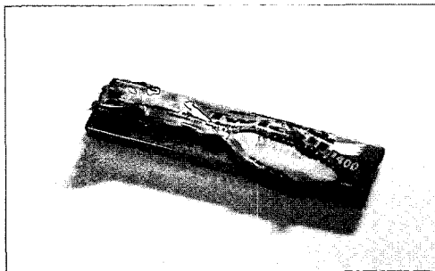
Fig. 14. Failure of slim type rechargeable cells due to temperature rise
