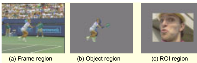
Fig. 8. Three regions where PSNRs are obtained in the simulation.
