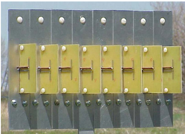
Fig. 8. Photograph of the printed dipole antenna array.
