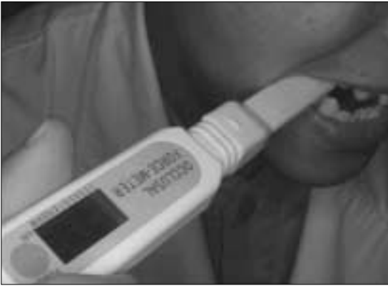
Fig. 5. The device for maximum bite force (Occlusal force-meter GM 10®)
