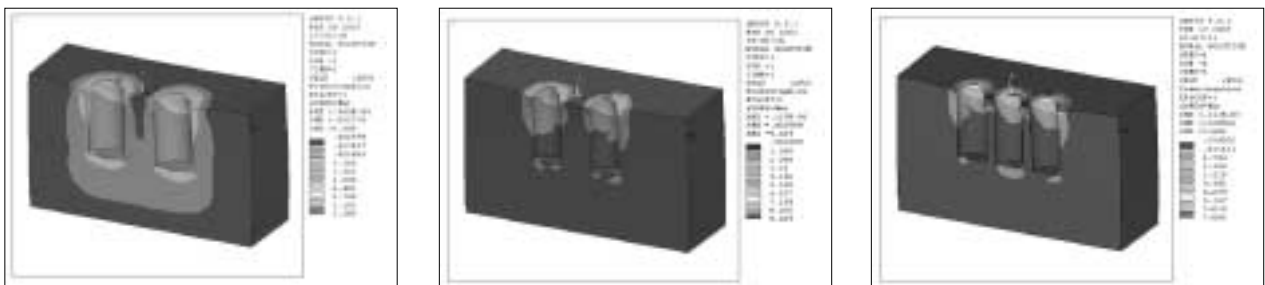
Fig. 4. Loading condition A : Distribution of Von-Mises stresses
